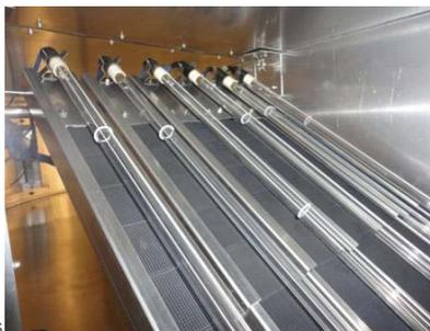
The UV-C light portion of the study simulated airstream microbe inactivation in an ASTM-/AHAM-style environmental test chamber that simulated a typical building's indoor environment and HVAC air-handler arrangement. A single-pass test was also performed on an ASHRAE Standard 52.2 test duct system.
