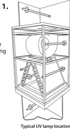
**Important:** some materials inside the air system (including filter media, flex duct, wiring etc.) may not be UV light resistant. Use the optional UV shield (part #TUV-SHIELD-LPC) or cover the materials with reflective tape.
