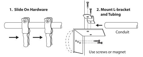
**2.** Mount the L-bracket and tubing as shown. Mount L-bracket to air handler wall using screws or magnet (galvanized metal only).
