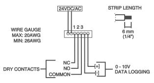
To remove a wire from the terminal block, insert a small slotted screwdriver (1/16" wide) into wire lock below the terminal and gently pull out the wire when it is unlocked.
