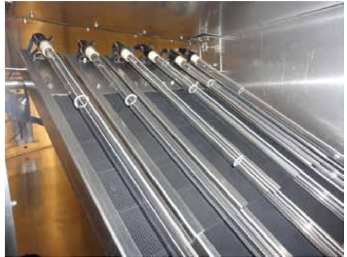
⚡ A 2012 study by Airmid Healthgroup actually proved UVGI’s effectiveness against mold, bacteria and viruses in a simulated HVAC-unit environment. The study simulated airstream-microbe inactivation in an ASTM-/AHAM-style environmental test chamber (shown here). AHG built the chamber to simulate a typical building’s indoor environment with an HVAC air handler, providing a 73°F (23°C) temperature, 55% RH and air-flow velocity of 492 fpm (0.93 m<sup>3</sup>/sec).
